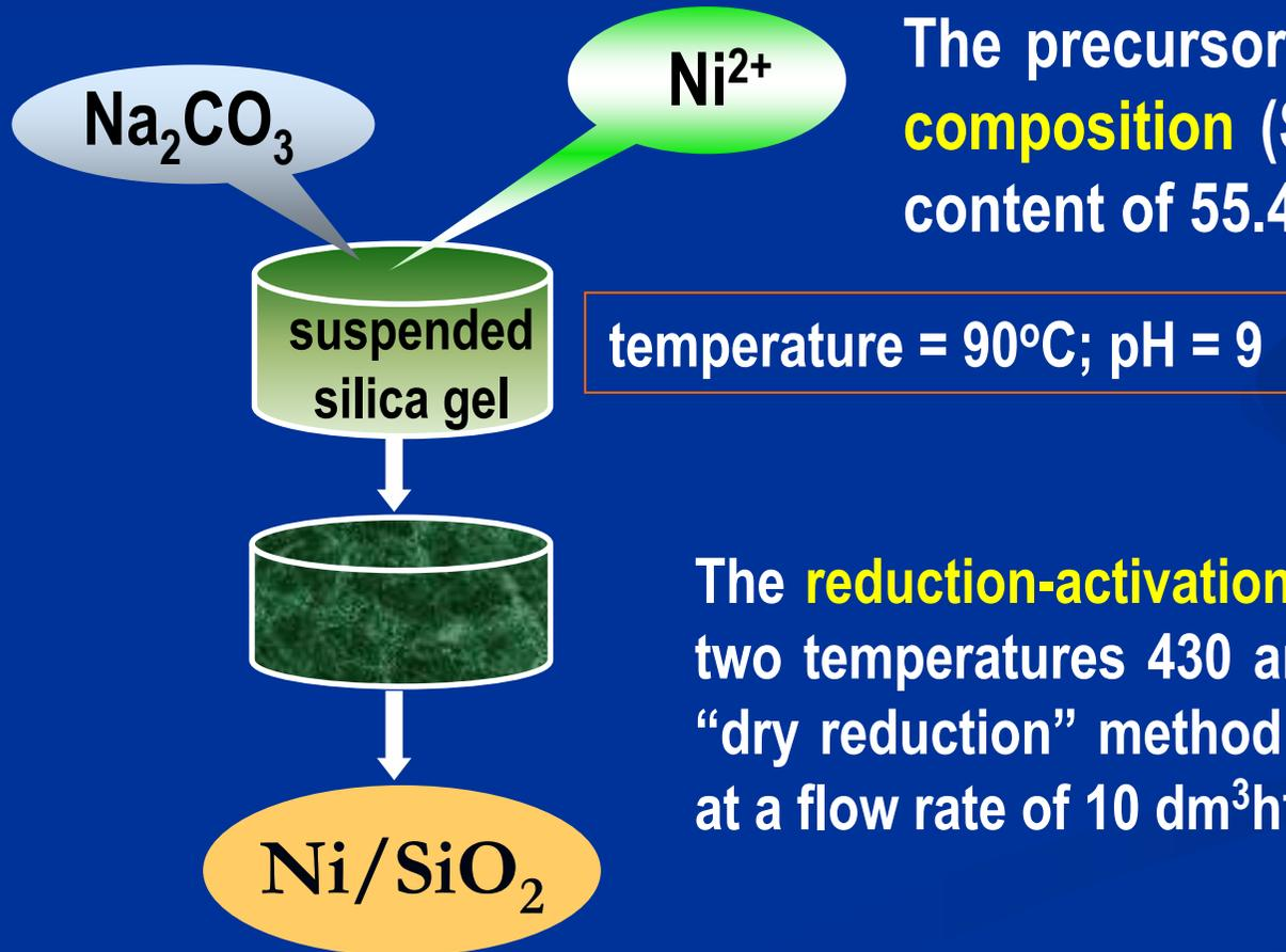
The **reduction-activation** of the precursors was performed at two temperatures 430 and 530°C in a laboratory set-up by a “dry reduction” method with a gas mixture of  $\text{H}_2/\text{N}_2$  (1/1 v/v) at a flow rate of 10  $\text{dm}^3\text{h}^{-1}$ .
