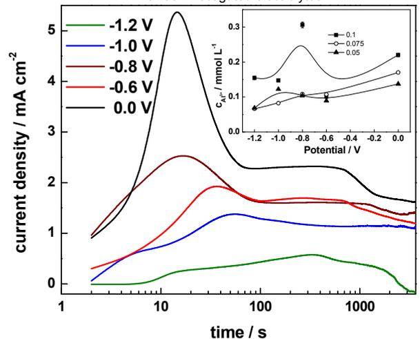
Fig. 3 Current density vs. time curves at different potentials in 0.5 M (NH<sub>4</sub>)<sub>2</sub>SO<sub>4</sub> + 0.1 M NH<sub>4</sub>F electrolyte; Insert - concentration of dissolved Al as depending on potential and fluoride concentration
