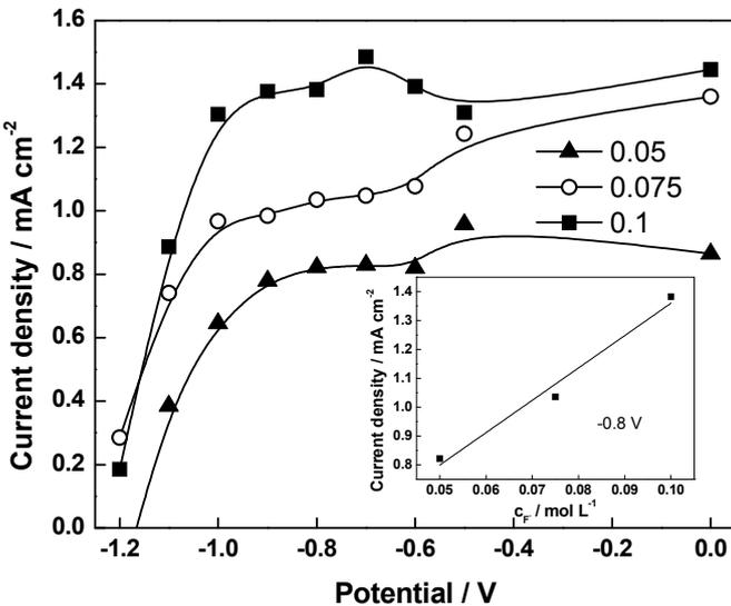
Fig. 1 Current density / potential curves in all investigated electrolytes in the potential range -1.2 - 0 V. Insert - dependence of current density at -0.8 V on fluoride concentration
