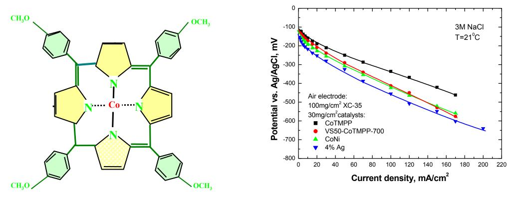
Polarization curves of air electrodes with
