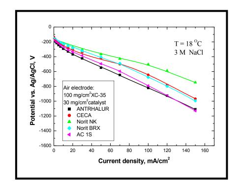
The observed differences in electrode characteristics are due to differences in the properties of the catalyst only
