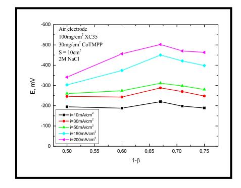
Current of the air electrode as a function of the catalytic layer content at constant potential
