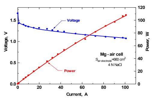
Experimental Mg-Air cell with 2 air electrodes (total working area of the air electrodes is 660 cm<sup>2</sup>) Current-voltage and power characteristics of the Mg-Air cell
