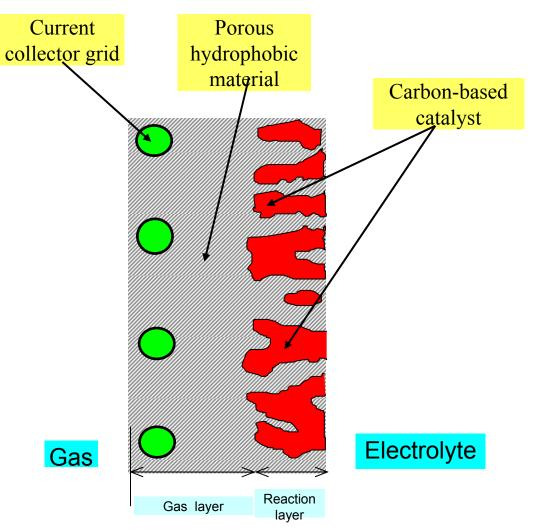
Effective oxygen supply for the catalyst Catalyst zones – no hydrophobic or binding agents
